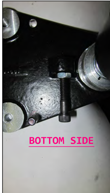
Fig. 37 Remove black screw with silver nut from bottom side of assembly and reinsert into top side of assembly.
