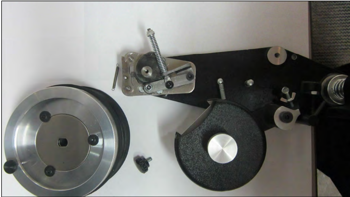
Fig. 11 Flip latch end for end & reinstall on opposite side spring pin.
