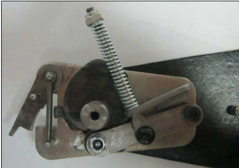
Fig. 8 Release tension from latch spring.
