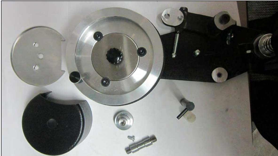
Fig. 31 Reattach extension spring from pivot arm to spring post and reposition pivot arm to other side of coder base plate. Secure with shoulder bolt using 3/16" Allen wrench.
