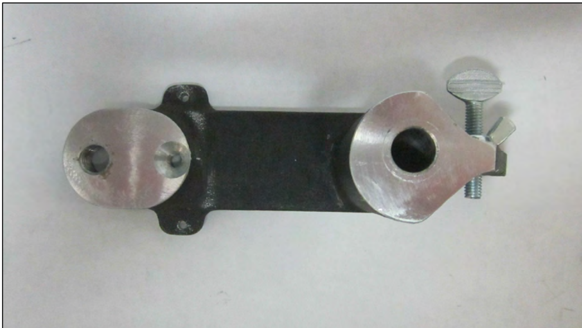
Fig. 26 Remove the thumbscrew and wing nut assembly from top side.
