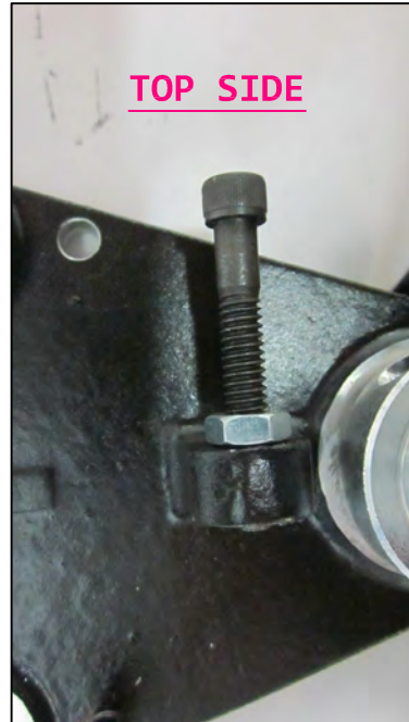
Fig. 37 Remove black screw with silver nut from bottom side of assembly and reinsert into top side of assembly.
