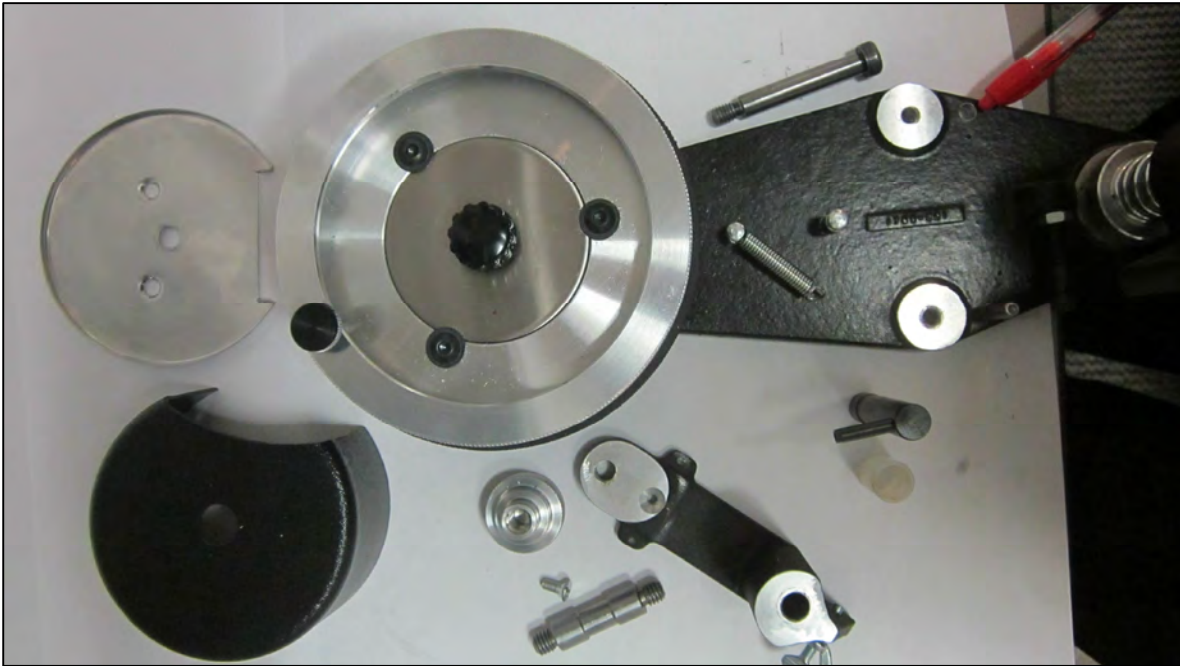
Fig. 29 Relocate pin in top side hole indicated by red pointer using a hammer.
