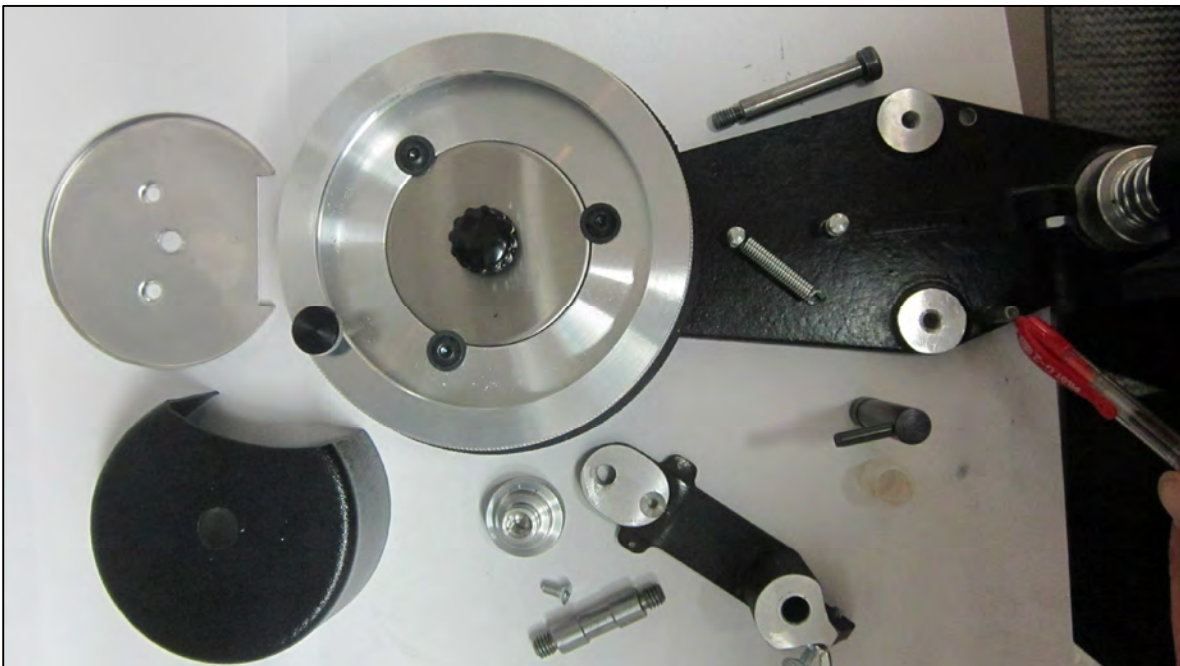
Fig. 28 Remove black cartridge cam & white sleeve from pin on bottom side. See (Fig. 1) Remove pin indicated with red pointer using a pin punch and a hammer.
