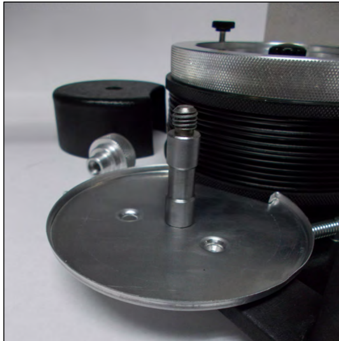
Fig. 20 Locate the ink roll shaft protruding from center of circular tray. Note the smaller diameter middle section of shaft.
